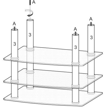
Screw long rods (A) into cylinders (3).
